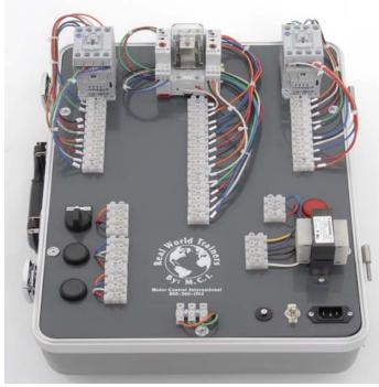
The Real World Trainers by M.C.I. are a set of five Motor Control Modules designed to teach Three Phase Motor Control using Single Phase 110 volts AC. The above module (RWT-D) maybe used to teach Low Voltage Motor Control, Relay Control and Timing Circuits. It may be used as a stand alone module. This module may be used with the other modules to teach more advanced timing and control circuits. All control circuits are hard wired using industrial standards.
