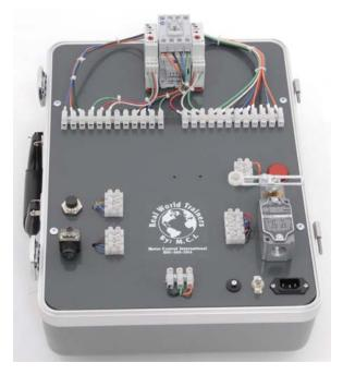
The Real World Trainers by M.C.I. are a set of five Motor Control Modules designed to teach Three Phase Motor Control using Single Phase 110 volts AC. The above module (RWT-E) is to be used with the other modules to teach Sensors and Timing Circuits. It may be used as stand alone as well. All control circuits are hard wired using industrial standards.
